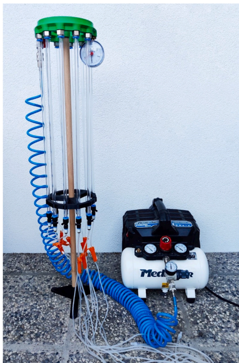
Fig. 1. Vertical PVC tubes for medium connected to a compressor.
